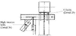
Beam-Column Connection for Truss Structure Example 18
